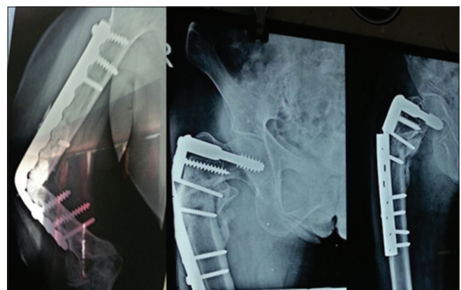
Figure 4: Plate failure in the humeral shaft and proximal femur
